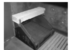
Burner with cast iron insert
